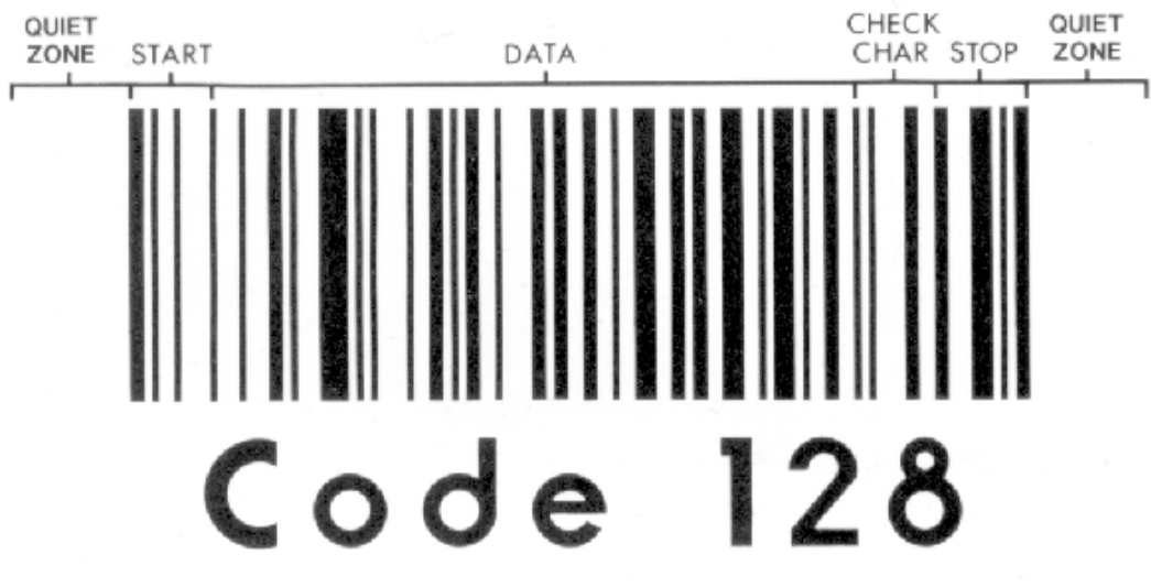
Figure 2.2. Structure of Code 128 with quiet zone
